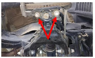
Remove the ball joint cradle bolts. Retain hardware.
