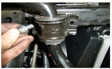
Install the ReadyLIFT sway bar brackets to the frame with the offset holes forward. Use factory hardware. Torque to 35 ftlbs.
