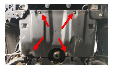
Locate the front driver and passenger side gravel guard mounts on the frame. Look to see if there will be any clearance issues with the front differential mounts when it is lowered. (Driver side shown.)
