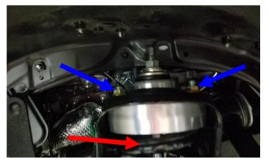
Raise the lower control arm up and install the OE lower strut hardware. Do not tighten at this time.
