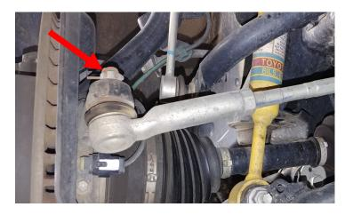
Strike the tie rod boss with a hammer to dislodge the taper. Remove the tie rod from the knuckle. Let the tie rod hang out of the way.
