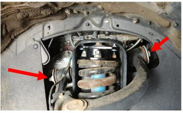
Install the lower ball joint cradle to the knuckle using the factory hardware, and a drop of thread locker. Torque to 125 ftlbs.
