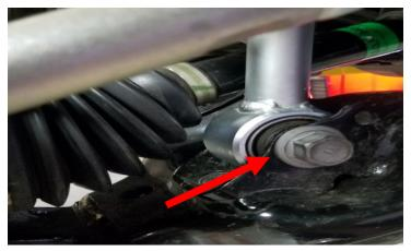
Loosen but do not remove the upper control arm hardware to allow the bushings to relax and have the suspension droop out. Make sure the CV axles do not over extend.
