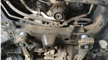
Install the previously removed driver side gravel guard support using the factory hardware. Torque to 45 ft-lbs. (Modified mount shown)
