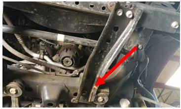
If so, mark the protruding area with a suitable marking tool. Remove from the vehicle and use a suitable cutting tool to trim off the marked section. Sand off any burs left over from the cutting. Use a quality rust-preventative paint on the exposed metal.
