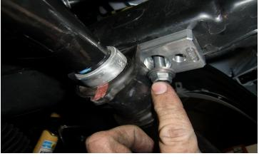
Install the sway bar to the ReadyLIFT brackets using the provided hardware. Torque to 35 ft-lbs.
